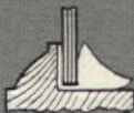
Ordinary putty takes on little resistance to shock, and soon may be easily broken.
