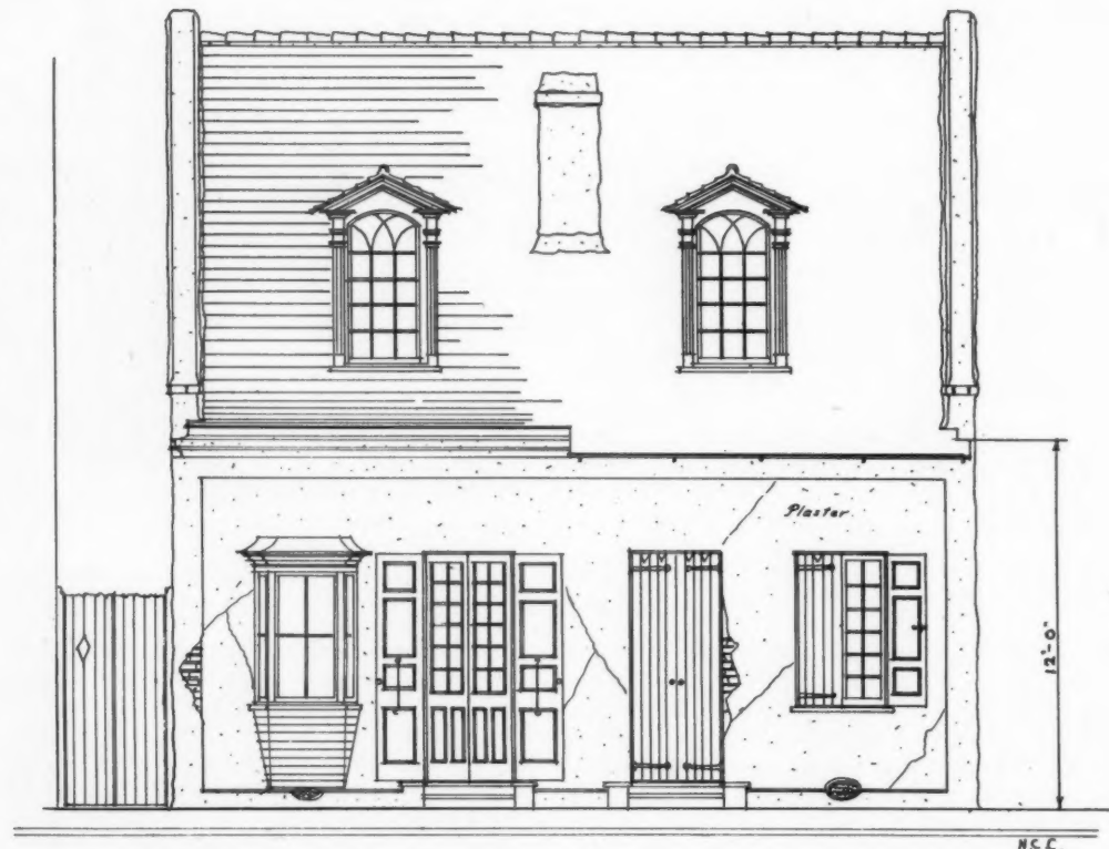
(ABOVE) TYPE OF SMALL DWELLING AND SHOP OF "BRIQUETTES ENTRE POTEAUX," CONSTRUCTION, PERIOD 1730-90 (BELOW) STREET FACADE OF A TYPICAL SMALL DWELLING AND SHOP IN THE "VIEUX CARRE," PERIOD 1750-1800
