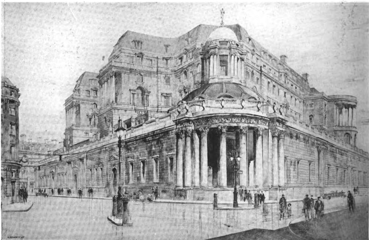
PERSPECTIVE AT LOTHBURY AND PRINCES STREET CORNER SHOWING SUPER-STRUCTURE ABOVE THE SOANE FACADE AND THE NEW DOME OVER CORNER
