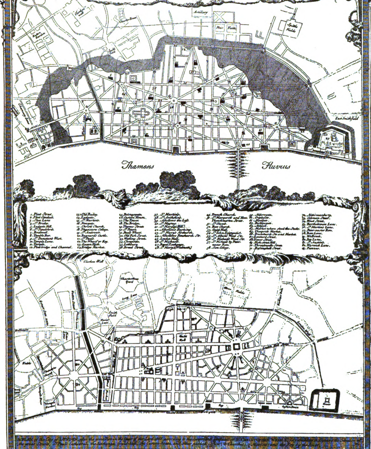
The second of two plates published by the Society of Antiquaries of London, dated 1748, showing John Evelyn's third plan for rebuilding London in 1666, and Wren's plan. Note: This plate was erroneously recorded on page 117, March issue.
