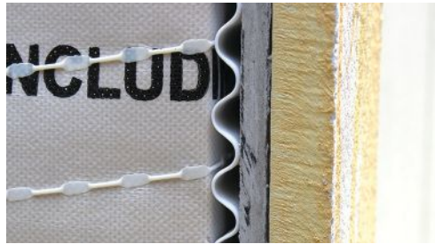
One type of housewrap on the market eliminates excess moisture from an exterior wall by providing drainage space between the housewrap and exterior sheathing. This is achieved by bonding very small spacers to the wrap. Photo courtesy of Tamlyn
