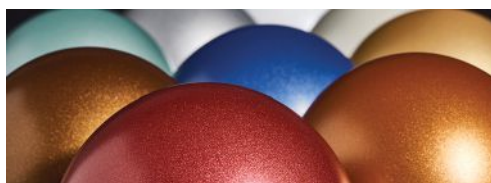
Metalescent pigments are composed of tiny metal flakes of aluminum, natural mica or synthetic mica-like material. They can produce coatings that shine and sparkle as a result of the size and shape of the metalescent flakes.
