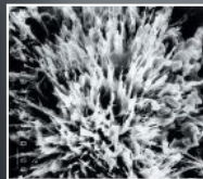
Xypex Crystallization (Mature)
