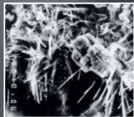
Xypex Crystallization (Initiated)
