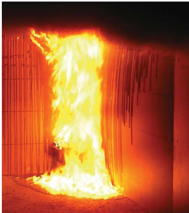
Standard NFPA 286 test method with HDPE untreated panels mounted on fire test room walls.
