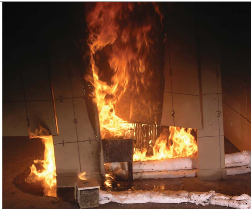
HDPE untreated panels being tested as they would be installed as toilet partitions in the field.
