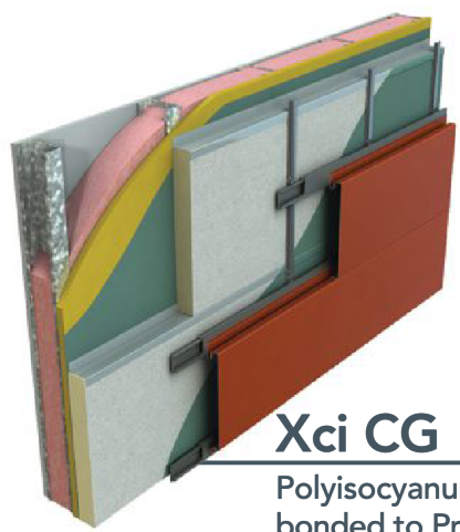
Xci Foil Polyisocyanurate Insulation bonded to Foil Facers
