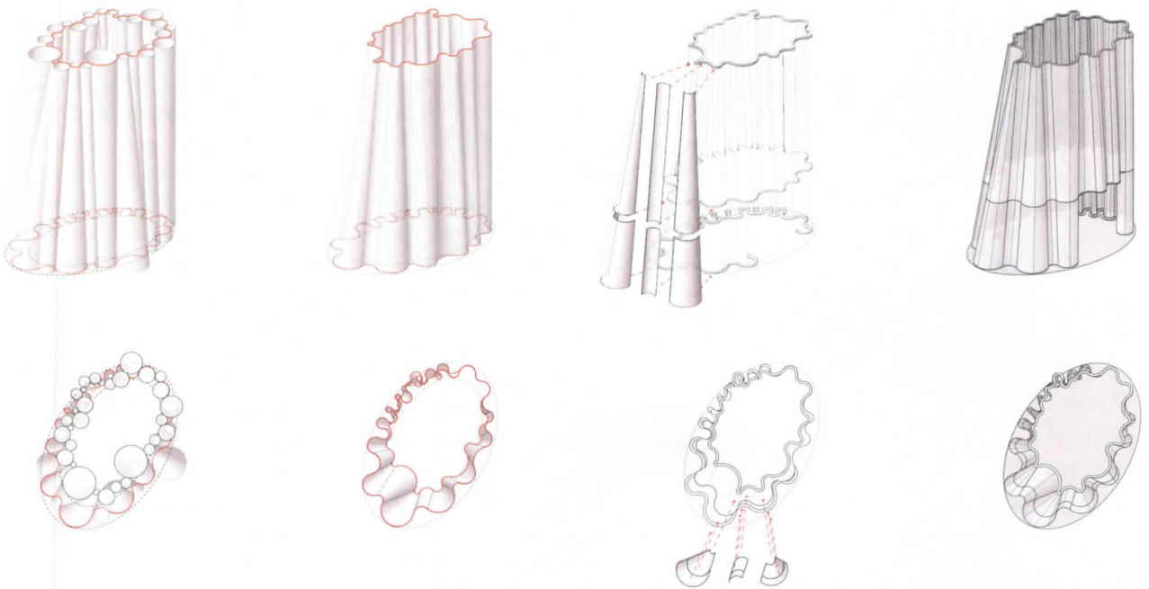
from left to right (top and bottom): bundled tube geometry, surface path, pattern assembly, assembled tower
