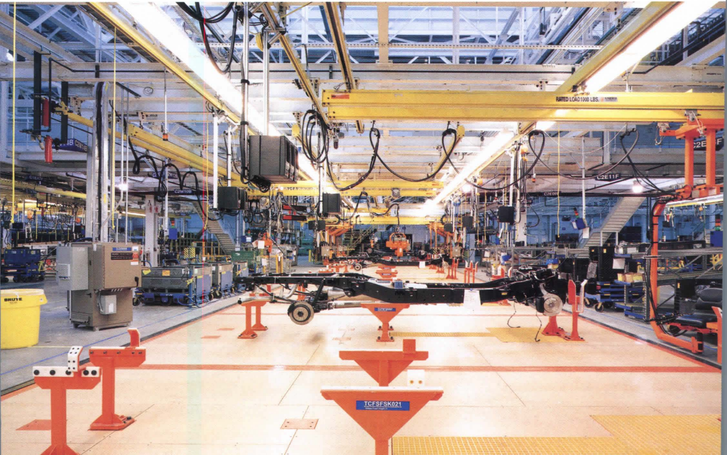
Beneath its 10-acre sedum roof (preceding pages) Ford's 1.16 million-square-foot truck plant is a lesson in structural and organizational choreography, with catwalks and ductwork hovering above 16 identified work cells dedicated to various assembly and testing functions.
