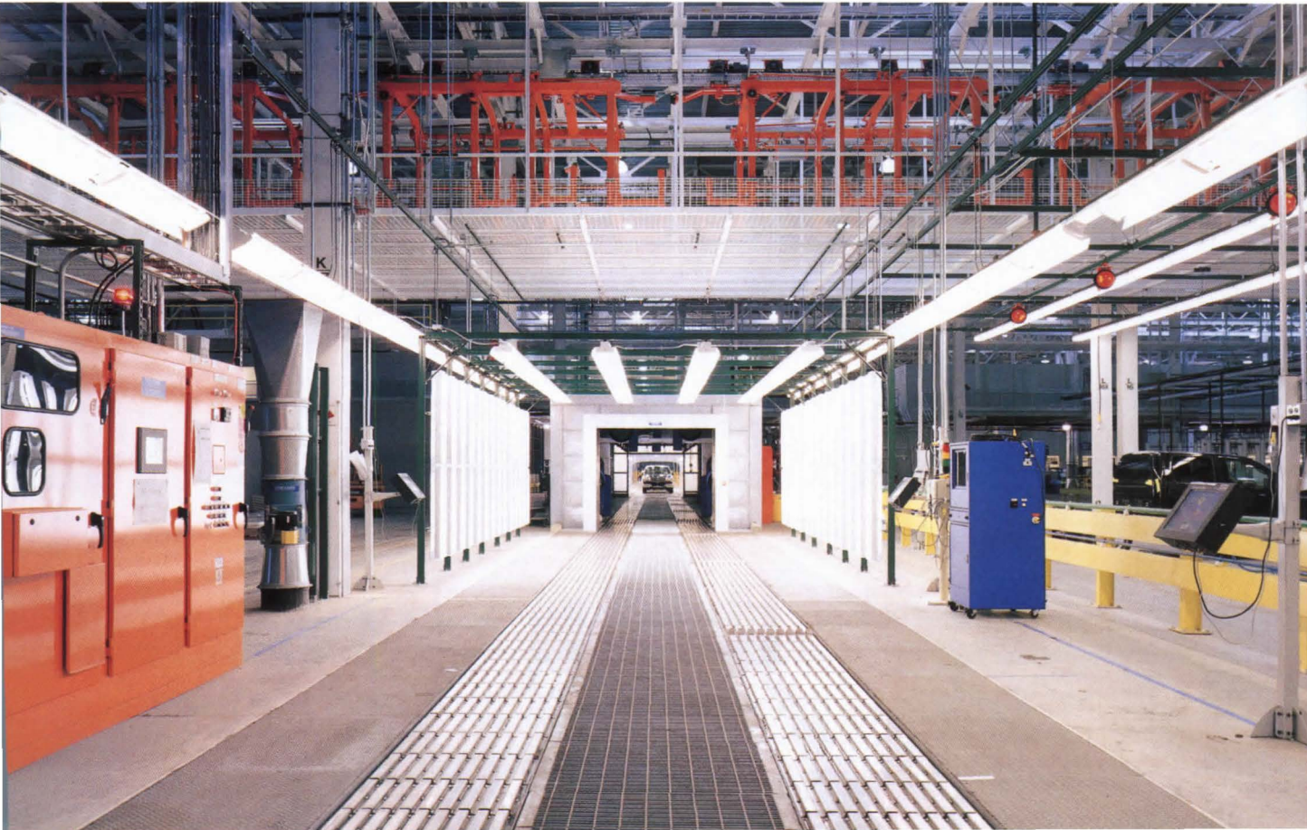
A web of truss work accommodates all matter of assembly needs, while massive light monitors reduce the need for artificial illumination. Ford employs "synchronous material flow" and waste-reduction techniques to help limit the environmental impact of their processes.
