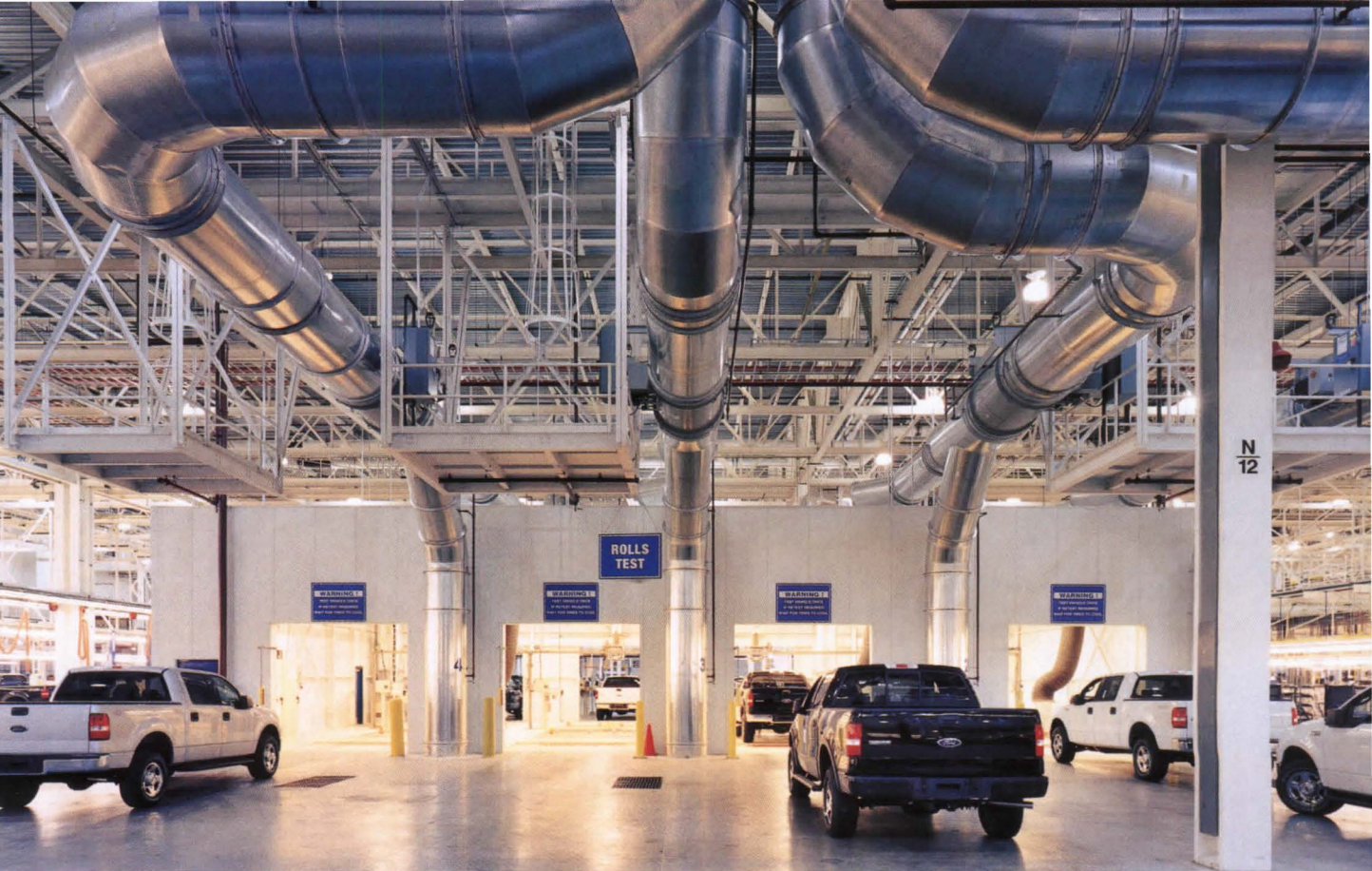
A web of truss work accommodates all matter of assembly needs, while massive light monitors reduce the need for artificial illumination. Ford employs "synchronous material flow" and waste-reduction techniques to help limit the environmental impact of their processes.
