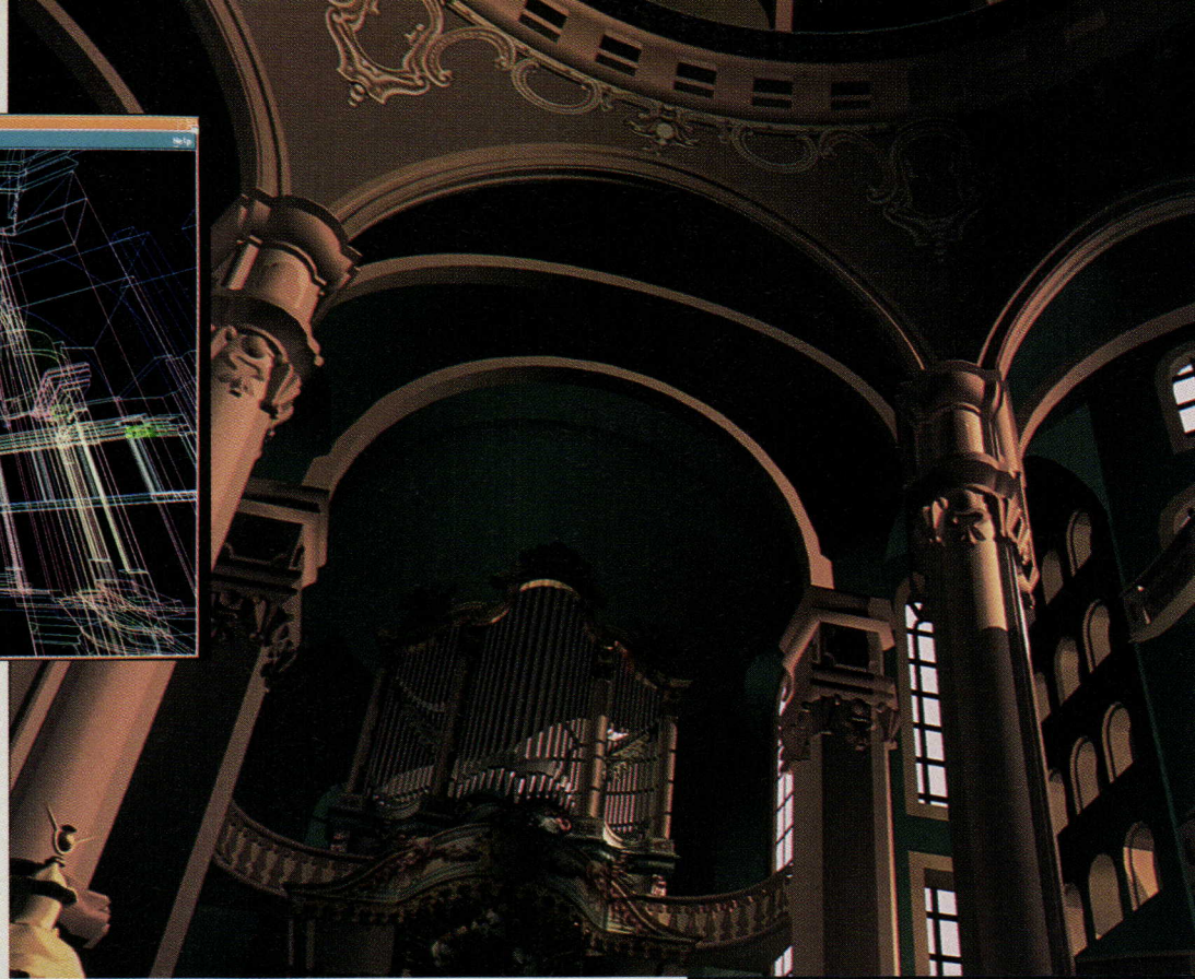
Wire-frame CATIA model (above left) and rendered 3-D virtual-reality model (above) document pendentives around dome.
