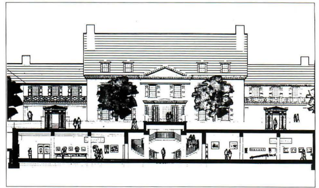
SECTION: Galleries housed under terrace.
