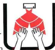
The ACCU-ZONE advantage—two zone-focused infrared transmitting beams create a large detection zone confined strictly to the bowl.
