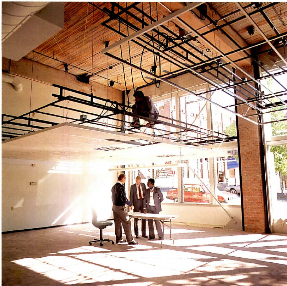
The 30-foot by 40-foot lab's mock-up potential ranges from a succession of spaces to a single office (above). The lab provides lighting fixtures for testing and advice to designers free of charge.
