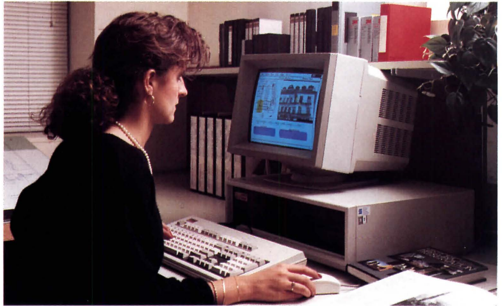
The typical OGS workstation (above) consists of a high-end personal computer—with an 80386 microprocessor and running at 20 MH, five specialty circuit boards, an internal hard disk of 130 megabytes or more for video and graphic records, an external optical disk drive and a modem and a laser printer. In-house and off-the-shelf software create facilities management reports (below).
