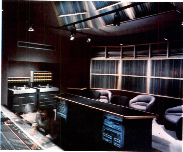
The control room of Tele-Image, Dallas, contains rear wall and ceiling diffusers for uniform listening throughout the room.
