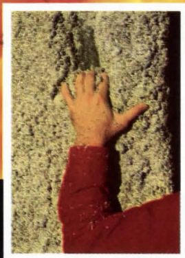
Mineral Wool Sprayed Fiber
