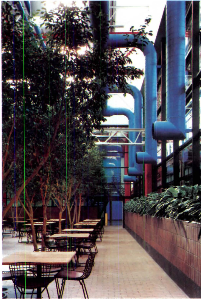
Red denotes structure, blue HVAC in the interior color scheme. Trees in dining area, left, filter natural light from above. Seating with built-in lights, right, snakes along L-shaped reception lobby, where visitors have views onto manufacturing floor. White wall, below, serves both as light reflector from hooded, linear skylight and as sound baffle. □
