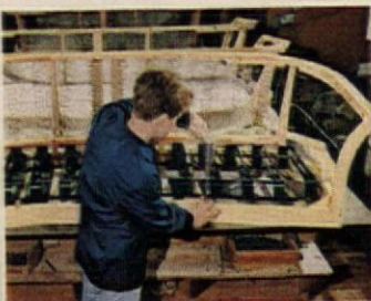
Lifetime springs are permanently attached to the solid, kiln-dried hardwood frame. Frames are double-doweled, not just glued.
