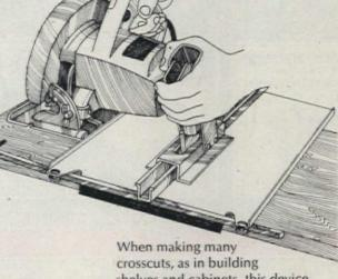
crosscuts, as in building shelves and cabinets, this device can save time and assure accurate work. You place it on a board up to 12 inches wide, place its set-up bar on your layout mark, then squeeze the handle. The Sure Square grips the wood to serve as a firm guide for a straight, accurate cut. Works with hand circular saw, saber saw, or router. Costs \$13.50 from Independence Specialties. For \$1.50 more, you get a kit that adapts the tool for drilling shelf clip holes.
