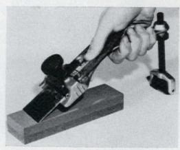
Chisel Sharpener, and is offered by General Hardware for \$4. To use, clamp the blade or chisel into the device, then rub the cutting edge over an oil stone as shown above. Since the blade cannot rock, you get a perfect edge every time. Bevel angle is adjustable.
