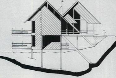
Drawing shows structure lifted above ravine, eliminating need for excavation and expensive foundation. Concrete piles of varying heights accommodate house to rugged site. Long diagonal wood brace is attached to buried concrete "land anchor."
