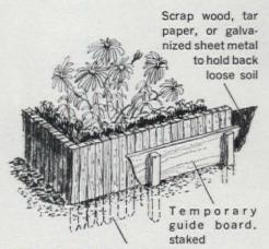
Drive in rough wood stakes, 2x2x18" long, about ½ length in ground. Keep tops level
