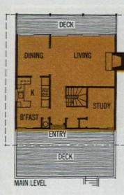
This two-story design overcame the problem of an unusually steep site by using a foundation of poles 12 inches in diameter on concrete footings. The high peaked roof has glass gable ends above the living room. The living area is expanded 50 percent by the decks to which six of seven rooms have direct access. Shingled walls fit in well with the wooded site that has a view of San Francisco Bay.
