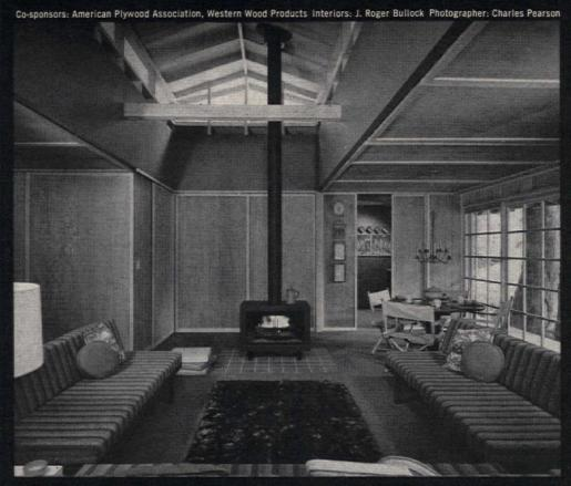
Combination box beam and half-truss roof system create clerestory. Hinged ceiling panels drop down (above and right) to form three additional sleeping areas. Kitchen is in rear. Even with hinged panels lowered there is plenty of living space. Plan shows that most of house is devoted to living areas. Weather tight in one week, construction costs were about \$7100.
