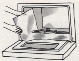
These are aluminum foil linings for the sides, top, and bottom of the oven. When they get soiled, don't scrub... just replace them with standard 18" foil available at most stores. This is an easy way to keep your oven clean.
