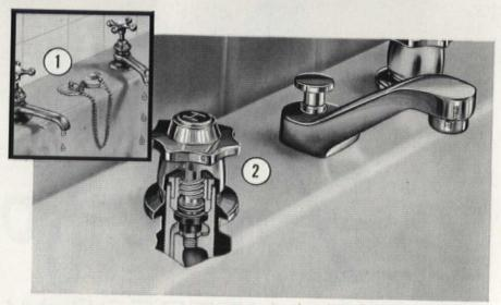
With every turn of the conventional faucet, (1) mechanical friction is applied to the washer . . . quickly wearing it down and allowing water to leak through. The AQUASEAL (2) operates by water pressure, which eliminates friction and wear . . . ends leaks and washer replacements.
