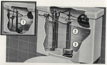
As the chain or rod (1) in most toilets becomes worn, bent or broken, the seal fails to seat properly, and water continues to run. Because the sleeve (2) of the new American-Standard flushing mechanism rides up and down on a stationary rod, it cannot slide out of position. Therefore, the seal (3) always provides a positive shutoff.
