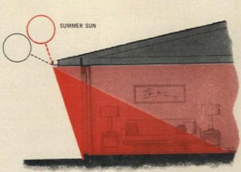
A roof overhang on a southern exposure shades windows from high summer sun but admits low winter sun. Depth of projection depends on the latitude of the house. Overhang will not protect against low east and west sun. These exposures can be shaded with planting or fencing.
