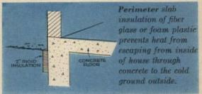
Concrete slabs laid on the ground almost always feel cold underfoot if not correctly insulated. The easiest remedy is to excavate around the outside of the foundation walls and apply rigid, 2-inch-thick, waterproof insulating boards tight against the walls. The boards should extend from just above the level of the slab to a depth of at least 12 inches.
