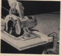
**Cut plywood** accurately with a portable circular saw by guiding the saw with a straight piece of wood clamped to the plywood.
