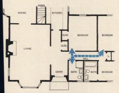
**Bcd placement of bathroom.** An embarrassing result of bad planning is this situation where a bathroom that serves two bedrooms is completely exposed to entry and living room.
