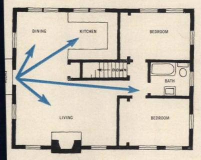
**Poor planning ruins privacy.** Open planning, which is so necessary to give a feeling of space to small houses, was poorly done here. Each area is exposed to the front entrance of the house.
