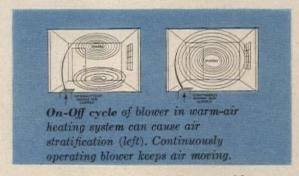
eliminate air stratification and thus provide more even temperatures at all times in all rooms. If the heating plant is too small, you can install an auxiliary plant for the rooms far removed from the central system—say, electric or gas wall heaters, a gas or oil-fired floor furnace, or radiant panels in the ceiling. Or you can rebuild a fireplace with a prefabricated metal firebox that circulates the heated air within the room and even to adiacent rooms.
