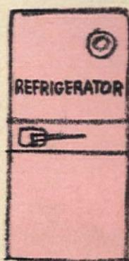
**WHEN REFRIGERATION FAILS** check *electric* refrigerator to see if it is plugged in or if house fuse has blown. Make certain pilot is lighted in *gas* models. Check control dial.
