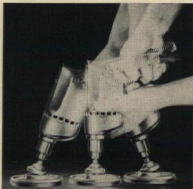
**NEW SANDER ATTACHMENT** for  $\frac{1}{4}$ " and larger electric drill chucks has a flexible ball-joint that lets you hold the tool at the angle you want, yet permits gouge-free sanding. The tool can be used on furniture, painted surfaces, and for cleaning and smoothing metals.
