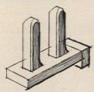
A TWO-HANDLED, "HOLD-DOWN" stick should always be used when you are cutting deep dadoes or grooves in a piece of wood. This will hold the work securely without endangering your fingers while you pass the work back and forth across the circular blade.
