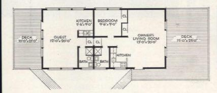
EXISTING PLAN shows doorway between guest and owner's section, flanked by closet space when units are used separately. Fold-away closet door permits traffic through hallway from one area to the other when entire house is used by the owner.
