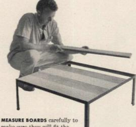
**MEASURE BOARDS** carefully to make sure they will fit the top snugly. Cut boards a triffe longer to allow for sanding.
