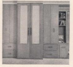
METICULOUS DESIGN of this storage unit, built across one wall in a master bedroom, makes space for everything in a man's wardrobe. Pull-out drawers for fold-up clothing are on the left, bulkier clothing in drawers on the right. Center space has built-in dressing section with lighted mirror, drawer for accessories and space for hanging sport shirts below. When closed, the unit makes a handsome and architectural feature of the room. (continued on page 81)
