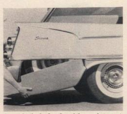
Spare tire in fender. Out of the way but easy to get to. Lets you fix flats without unloading cargo.
