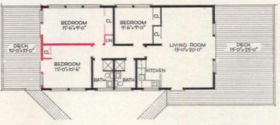
ALTERNATE FLOOR PLAN shows simple change required where more bedrooms are needed. Plan in red indicates changes. The two bedrooms added each have access to deck; high windows allow for flexibility in arrangement of furniture against wall areas.
