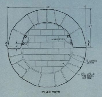
A small barbecue only 5 feet in diameter with big barbecue performance. Large counter-high semi-circular wind-wall makes excellent working counter. It will fit into almost any yard. Here's how to build it:
