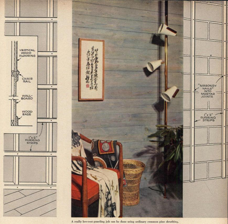
A really low-cost paneling job can be done using ordinary common pine sheathing. In this particular instance the wood was given a driftwood finish. When paneling is to be applied over a masonry wall, the wood furring strips must first be applied to provide a nailing base for the paneling. Furring may be fastened to the concrete with cut nails, masonry anchors or with special adhesives. Lumber stock is usually a regular 2x2" size and is quite suitable for use as furring.
