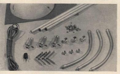
ere's a modern floor lamp with three gooseneck-mounted lights that make it a really flexible lamp. It requires few tools and little work, uses an assortment of easy-to-obtain parts, including: wood salad bowl, 11" in diameter; tempered hardboard, 1/8" thick; 3 lengths of 1/2" thinwall conduit, 35", 38" and 41" long; 3 conduit connectors; 3 flexible goosenecks; 3 lamp sockets; 3 or 4 small angle irons;
