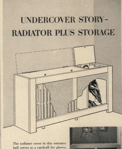
packages and such etceteras. The compartment in one end of cover provides storage for muddy rubbers and wet umbrellas. Tops on storage compartment and radiator lift back for easy access to their interiors.
