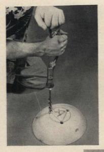
Make the lamp base from a salad bowl. First remove wax finish, using coarse sandpaper, and drill three 3/4" holes in the bottom of bowl at equidistant points around the 4-inch circle. These holes receive the 1/2" thinwall conduit. Connectors are tightened on conduit ends before putting on hardboard bottom.
