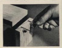
To drill blind dowel holes put two finishing nails between two pieces of wood; anchor nails with putty. Nails leave marks used for drilling centers.
