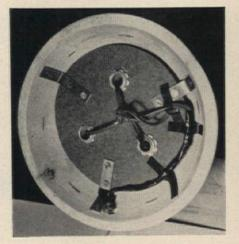
Bottom view of base shows hardboard disc secured by screws, stove bolts and small angle irons bent to curve of bowl. Attach goosenecks; connect light sockets with lampcord; thread wire through lamp; splice to main wire; for wall outlet, connect plug.
