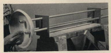
To align uprights, make a temporary support of two 6x6" pieces of hardboard with 34" holes drilled in the same position as they were in bowl bottom; nail 6" pieces to ends of a 24" length of scrap board or plywood. Slip conduit uprights through the holes.
