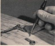
One quick and easy way to make a starting hole for a screw eye or a small screw is to punch a hole in the wood with a slender nail-set instead of drilling it.
