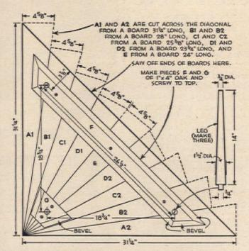
Sketch of underside of table shows sizes and position of pieces.
