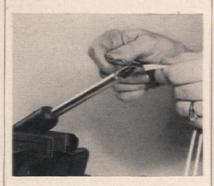
Vise can be your third hand when doing small soldering jobs like joining electrical wiring. Grip iron in vise, hold work on iron; touch with solder when it's hot.
