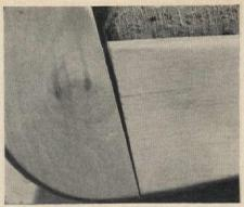
When the joints in the arr legs, back or seat of yo chair loosen, they sques Repair the loose parts qui ly or you may end up w little more than a heap kindling. At left is a typic joint separation where g holding doweled joint bro up and pieces pulled apa
