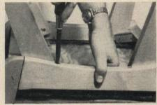
The first step in compl reglueing and repairing chair is to remove the s This is done (on most chai by turning the chair ups down and removing down and removing screws which are coun sunk in the chair frame si
