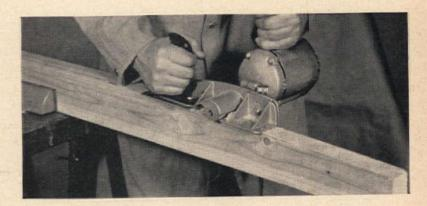
Roof members of contemporary model taper slightly at front ends to give a professional appearance. Unit plus circular saw makes rough cut, then planer attachment on same unit smooths, straightens, and squares up the taper. Finished wood behind planer and unfinished wood ahead point up effectiveness.
