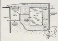
Plan view of pool plumbing shows position of water-supply pipes, filter tank, and pump under sun deck. Fresh water enters pool through two inlets in pool wall, and it returns to filter through drain in floor. Drain piping must be installed before the floor is poured. The overflow from gutter is drained to a dry well at lower right.
