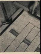
Miter ends of the two 6 lengths quarter-round; fas glue and 1" finishing edge of frame to form for panel. Glue surfaces angle rabbet, lay in pat then secure with quarter
