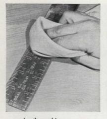
Are the markings on your square dimmed by time and use? You can restore their readability if you just dip a piece of cloth in light-colored paint and wipe the scale with it. The punched-in marks and numbers pick up paint, but rest of scale does not.
