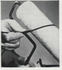
When you finish a roller painting job, you'll be able to salvage more paint off roller if you scrape the curved surface with the hook section of a wire coat hanger, as shown. It saves paint and it makes shorter work of the final cleaning of paint roller.
