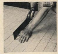
Begin by making pencil lines 4" in from long edges of panel. Then starting at center, draw lines across panel, 3" apart up to 6" from the end. Start cutting lines by working cross-cut or back saw back and forth till teeth dig in.
