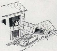
the sides and rear, 3' above the ground. The roof has 2" by 4" joists at 4' intervals, topped by rough 1" boards and asphalt roll roofing. The corners are braced with 2" by 4"s. The structure is painted green to match the roofing. It's doing its job and looks well, too.
