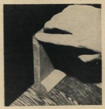
Fit a short length of wood dowel over tip of your bit to guard it from damage by other tools. Drill pilot hole in dowel with small drill to prevent splitting when screwed onto the end of bit.
