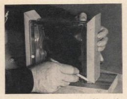
3. Hold block in place on teakwood base, with measurements even all around. Put the side pieces in place on base, and mark positions with pencil. Bevel all edges of the base 15° before you proceed to the next step shown.
