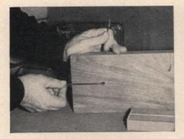
2. Drill  $\frac{1}{4}$ " hole in teakwood base directly under the groove in one of the side pieces. Then cut  $\frac{1}{4}$ " dado from hole to end of base on the underside. This will accommodate the electric cord. Bottom of base is shown in this view.
