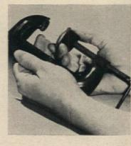
Fit a furniture glide (metal piece made for use on bottom of a chair leg) over tip of the screw on your C-clamp. It keeps screw from gouging wood held in the clamp, and holds work firmly in place.
