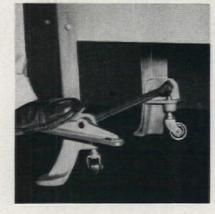
Miter gauge clamp holds work firmly. For wide work, screw wooden extension to miter face. To cut duplicate pieces, clamp a block to extension, as shown.
