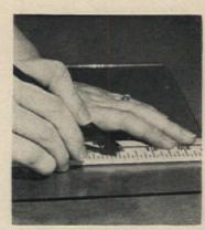
You can make glass-cutting easier and more accurate if you use a dampened yardstick as a guide for the cutter. The damp surface will keep yardstick from slipping as you draw cutter along its edge.
