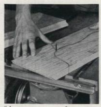
Saber saw accessory cuts fancy curves, saves cost of motor and table; can be used with miter gauge and fence, but it does not fit every make of saw.
