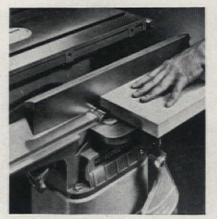
A jointer (can be added to most saws) cuts rabbets as shown, planes boards flat, and trues up and squares edges an essential for good cabinet work.
