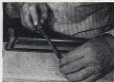
To file teeth, hold saw in clamp or between two boards in a vise. Use triangular file straight across on rip saw; at 45° angle on cross cut. File into every other gullet so that half of flat jointed top is filed away
