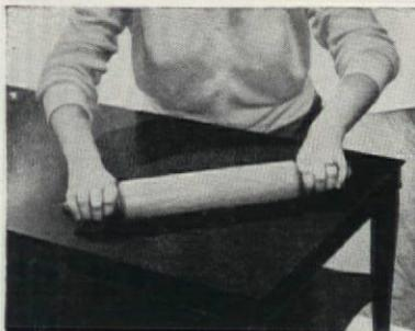
To assure a firm bond, roll the top from the center to edges with heavy pressure. Remove excess dry adhesive with solvent or with a hard rubber eraser.
