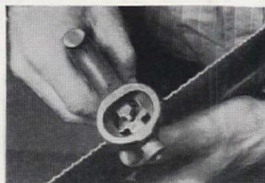
Set teeth to prevent binding. Start at one end with "saw set," which bends out every other tooth. Reverse saw. Set other half of teeth so that alternate teeth will point to opposite sides of blade
