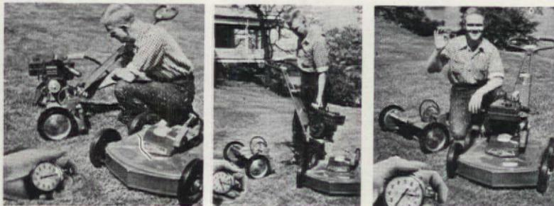
Timed by a stop watch, the "Power Handle" is transferred from a reel-type lawn mower to a rotary-type mower in just 20 seconds! A locking device makes the change from one unit to another a simple matter without tools. Since the handle itself and each of the basic units is smaller than a fixed-power unit, a minimum of storage space is needed.
