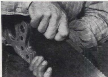
For a clean-cutting saw, all teeth must be uniform height, so first step is "jointing." With light strokes, pass flat mill file lengthwise over saw teeth until file just touches point of every tooth
