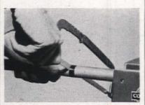
Wrap a piece of tape around a rod, tube, or dowel before cutting. Follow one edge with saw to get a perfect square cut
