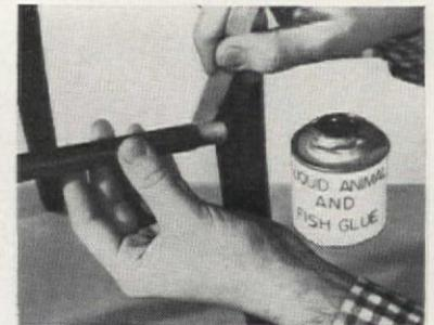
Liquid animal glue—for household repair and carpentry, makes light colored joint, will hold poorly fitted joints. It resists heat and mold, but not dampness. Apply it directly from container
