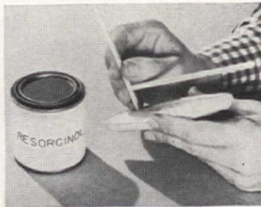
Resorcinol—for boats, outdoor furniture, other joints exposed to water or dampness, makes a very dark-colored joint. Use only at temperatures above 70° F., and mix catalyst and powder for each use
