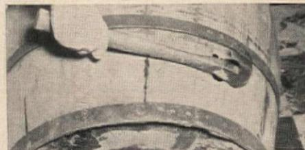
Then punch out centers with hammer (left). Be sure that staves and bottom are well nailed to hoops. Paint the barrel and, while it dries, get a piece of 4" stovepipe as long as barrel is high
