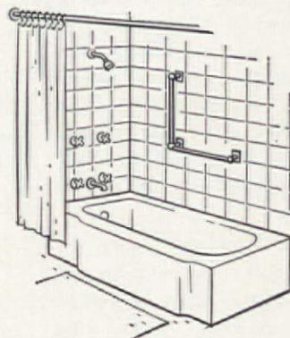
Come clean! Is your tub a security risk? To help prevent bad falls, install a hand grip of unbreakable material—a horizontal bar for the tub, a long vertical bar for the shower, or, as illustrated, an L-shaped bar for a combination shower and tub. Be sure it is firmly attached and easy for all members of the family to reach
