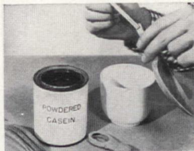
Casein—for cabinet work, heavy duty repairs, and for gluing oily woods, can be used at low temperatures, but is not completely waterproof. Will stain oak or acid woods. Mix fresh for each use
