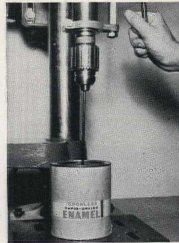
A special paint-mixing attachment is also available. To use it, lower mixer to bottom of can, lock spindle in this position, and operate drill press at low speed. Hold can to avoid spilling paint. Then move can around so mixer gets into the corners
