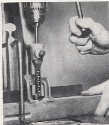
Mortising attachment cuts square holes used for good wood joints. Special fence has hold-down to hold work firmly on table. Depth gauge controls depth of cut
