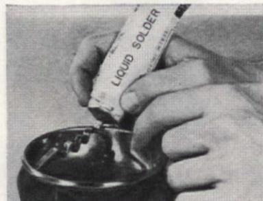
Liquid solder—for cementing metal, wood, or glass, is ready to use from tube, dries quickly, but leaves a noticeable metallic joint. It holds less well on wood than do other types of adhesive
