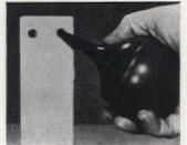
Small syringe sucks out chips and dust when used for cleaning a blind hole or crevice
