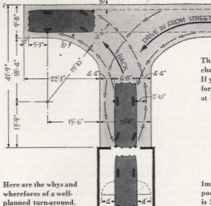
planned turn-around. The minimum distance from outside face of garage to far side of
