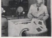
ATOMIC TESTS used Geiger Counter to accurately measure amount of dirt removed from cloth impregnated with radioactive soil.
