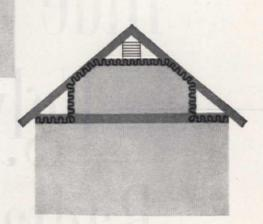
If attic is used for living, insulate around the rooms, leaving ventilated area above to prevent condensation
