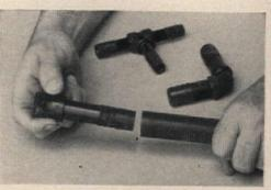
You can even buy kits for watering your lawn. These come complete with pipes, sprinkler heads, tees, ells, and an adapter to connect the system to an existing outside outlet
