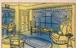
**CONVENTIONAL** heating or air conditioning methods try to combat unpleasant temperatures *after* they enter the room. Result: drafts (blue, above), uneven temperatures, poor circulation for freshness.
