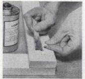
Glue wood plugs in holes over the screw heads to hide them. Also, countersunk screws can be covered with wood filler sanded smooth
