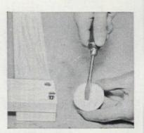
Screwdriver blade drawn across blue marking chalk, slips less in slot. Be sure to use a blade as wide as screw-head slot
