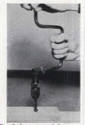
For flush or concealed screws, countersink with brace and bit, or cut wood plugs for later concealment of screw heads
