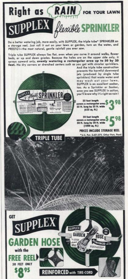
So light you can pick up 50 feet of hose with one finger, reel and all. Yet so tough you can actually shut it off at the nozzle and leave it under full pressure in the hot oun for days! That's SUPPLEX GARDEN HOSE,—all plastic for light weight and TIRE-CORD REINFORCED for greater strength.
