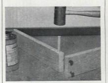
When driving screws in end grain, drill a hole near end of board, and plug with a tight-fitting glued dowel for extra strength
