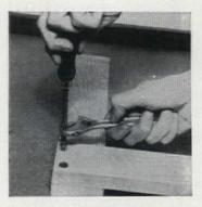
Hold screwdriver firmly in slot. For heavy work or long screws, a brace and bit, and even a wrench can be used for extra leverage
