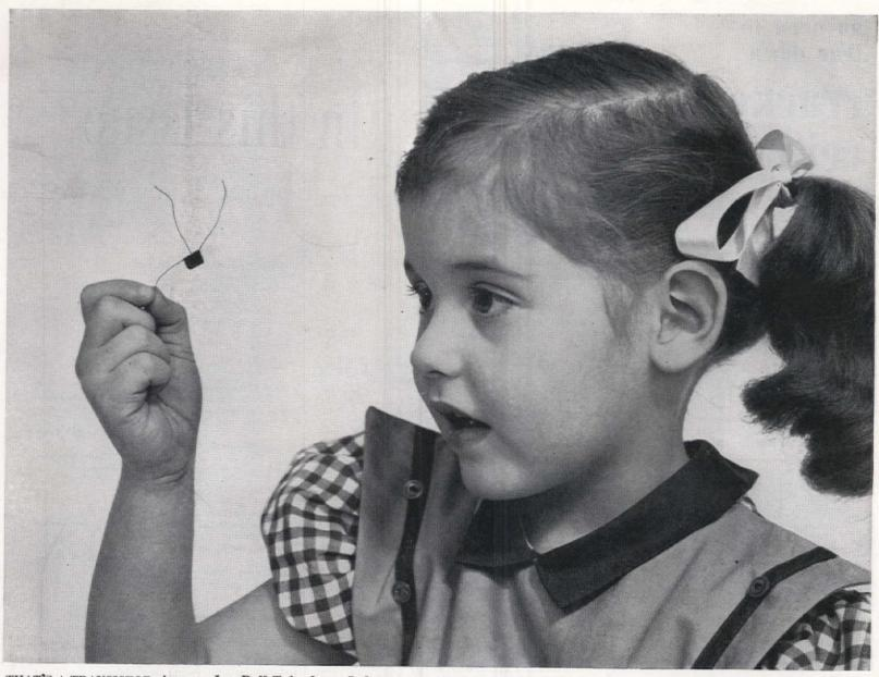
THAT'S A TRANSISTOR, invented at Bell Telephone Laboratories. This tiny electronic device can do many things that vacuum tubes can do and more besides. Though little larger than a coffee bean, it can amplify electric signals 100,000 times. Requires so little power that a coin, wrapped in a piece of dampened paper, can generate enough electricity to make a Transistor work. More than forty types of Transistors have been devised at Bell Telephone Laboratories.
