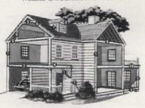
1. Exterior walls. 2. Floor above unheated garage. 3. Floor above unexcavated area. 4. Floor over open porch. 5. Ceiling below unfinished attic. 6. Sloping ceiling. 7. Dormer cheeks and faces. 8. Dormer ceiling. 9. Knee walls. 10. Ceiling below
