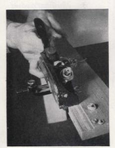
Frame consists of four short and four long pieces of 1 x 4 lumber. Shorts are width of opening, less 33/4 in. (width of lumber). Longs are length of opening, less 334 in. With plane or power saw, cut rabbets along edge of the four pieces. Rabbets should be 1 in. wide and equal in depth to the thickness of plastic used
