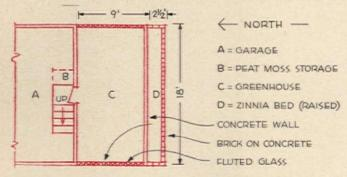
deep. As far as economical heating goes, the "sunken greenhouse" arrangement is very satisfactory, the garage protecting it on the north and partly on the east. Shoveling sand in from a trailer has been no trouble, but handling flats has been hard, as I have to carry them upstairs and around the front. So I plan to build a roller-type conveyor
