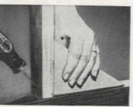
It's always difficult to toenail light pieces of wood without having them slip out of position. Try backing them up with a block of wood with a piece of rubber stair tread tacked to its bottom
