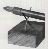
Make a serviceable soldering-iron support by driving two large finishing nails into a three-inch square of wood so that they form an X to hold the iron's tip
