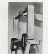
If you're taken with acrophobia when perched on a stepladder, provide yourself with a good handhold by building a sturdy square of lumber and clamping it to the top of the ladder
