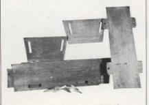
lengths of 3/8" maplewood dowel. Coat each piece of dowel with waterproof glue, then drive into tenons on floor of box. This prevents tenons from splitting when pegs are driven in. Assemble sides to bottom. For snug fit, you may find it necessary to file edges with a square rasp.
