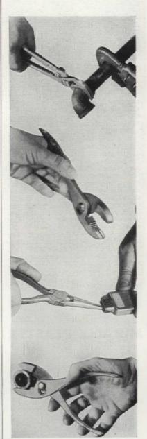
Water-pump pliers are good for many plumbing jobs, but should not be used on plated metal as they will scar the finish. As the jaws are expandable, they can be used on many sizes of pipe
