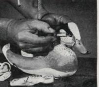
Assemble harp and socket base. Attach cord, fasten socket back in base. Pull out wire to eliminate slack. Add shade, remembering that rough fabrics like burlap, or the grasses, are best. You've now decoyed a mighty handsome lamp
