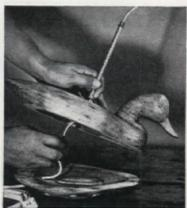
Pass cord through the base and then through the lamp rod. Knot cord to prevent it from slipping. Glue sections of decoy together, and further secure with wire brads, countersinking, and then filling holes and bad spots with plastic wood. Sand smooth when dry. Shellac, then paint decoy with flat white, and pencil in design when paint is hard. (For details of refinishing, see page 114)
