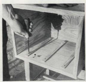
In order to locate slides on drawer housings, use try square to mark location of dados cut in drawer side pieces. Then install  $\frac{3}{4}$ " x  $\frac{1}{2}$ " x  $\frac{12}{9}$ " drawer slides as shown. Slides are fastened in place on drawer housings with two wood screws, as shown
