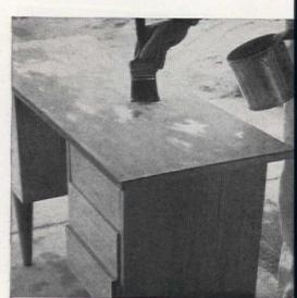
If opened grain wood has been used for desk, seal pores with wood filler. When filler is dry, sand surface smooth and apply finish of lacquer or varnish. Use several coats, and polish down with pumice stone and oil
