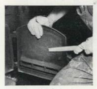
A warped ash pit or fire-box door on a coal-burning furnace can ruin its efficiency. It's often possible to make the door fit by filing down the high spots on the door edge
