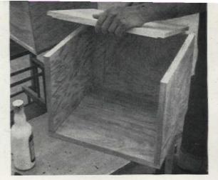
To hold the back, cut dado ¼" deep and ¼" wide along inside back edges of side pieces of drawer housing and top and bottom pieces. Drawer-box back is made of ¼" plywood, with outside veneer matching other exposed surfaces. Glue joints
