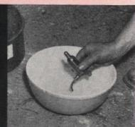
Steam radiators may fail to heat because air valve is stuck. Remove valve and soak in white gasoline which softens dirt and oil inside valve MORE PICTURES ON PAGE 110
