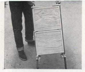
Assemble the two drawer boxes individually, or assemble both at the same time, as shown here. Use a piece of waste wood to protect the finished wood surface from the metal clamps. It is advisable to use four clamps rather than just two
