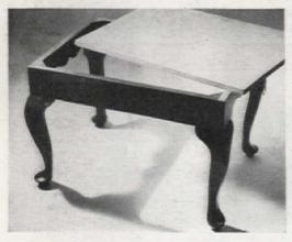
Make a "marble-topped" coffee table from any low frame, topped with 3/4" plywood panel covered in marbleized plastic. Cut plywood to fit frame top, coat with Fir-zite to "tame" grain. Fill nicks with wood putty. Dry. Rub with fine sandpaper
