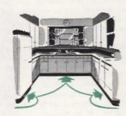
Best, most step-saving kitchen plan arranges equipment in a U. Ideal way is to progress from refrigerator on left, to sink, to range on right
