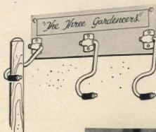
"Peg-Board" is device for hanging all sizes and kinds of objects in handy places. Sheets of brown Masonite (smooth or leatherwood finish) up to 48 x 96 in., with holes every inch, when screwed to studs (or, with 3/8" spacers, to flat walls) take bent ends of variety of hooks, brackets, clips (Peg-Board of New York)
