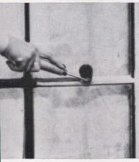
There is a roller made for working to edges and doing job mentioned above for the brush. It's shaped like a truncated cone and has a disc shield on the end. It works very well for window muntins and trim
