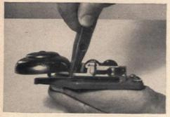
If the clapper doesn't strike the bell when it moves, bend the arm with small pliers. Adjust it a little at a time and test the tone of the bell after each adjustment
