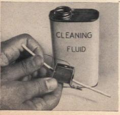
Dip a pipe cleaner in cleaning fluid and swab out the inside of the solenoid. Also clean the rod with the fluid. Reassemble the chime. Do not oil it. Oil isn't necessary and will catch dirt quickly. Clean the chimes once a year
