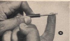
Be careful of the little spring that is on some rods. Its purpose is to return the rod to the original position after striking the chime, and it won't work properly if damaged in any way
