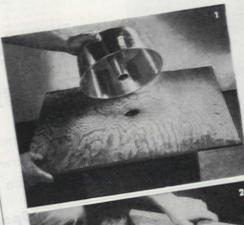
Cut a piece of plywood 4 inches larger on all sides than the base of your lampto-be. Cut hole in center to fit cone in angel cake pan. Oil outside of pan lightly, place as shown. (The base is made upside down-it's easier)
