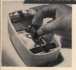
The electric circuit and its servicing are the same for chimes and bells. The operating heart of chimes is one or two solenoids and a sliding rod. Take the cover or back of the chimes off and remove the solenoid to clean it. In some models the solenoid can be cleaned without dismounting it
